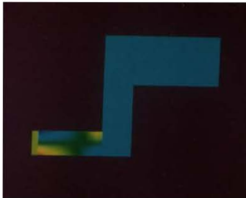
Figure 15. Radial Stress Fringes (S-Glass/Pin) Range: -189,000 psi - 309,000 psi
