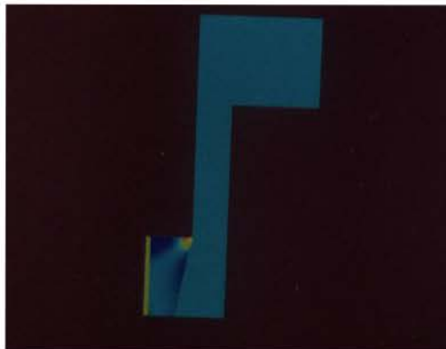
Figure 13. Radial Stress Fringes (S-Glass/Inconel) Range: -400 psi - 23,750 psi
