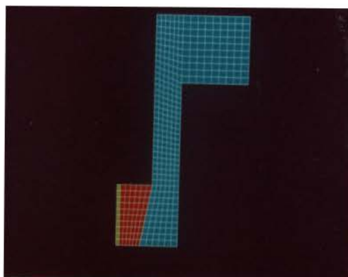
Figure 3. F.E. grid over color parts S-Glass/Inconel
