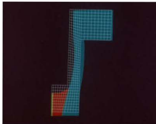
Figure 7. Deformed geometry (S-Glass/Inconel)
